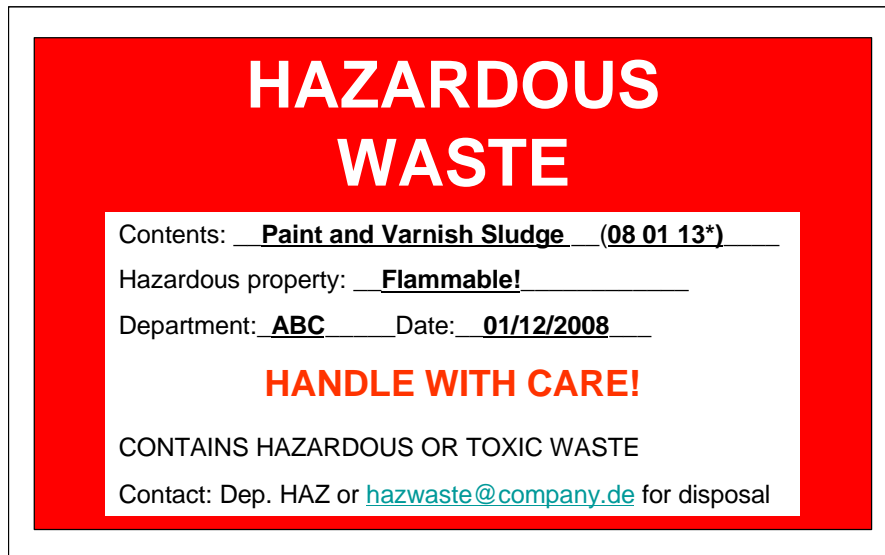
Figure 10 – Sample of a hazardous waste label
